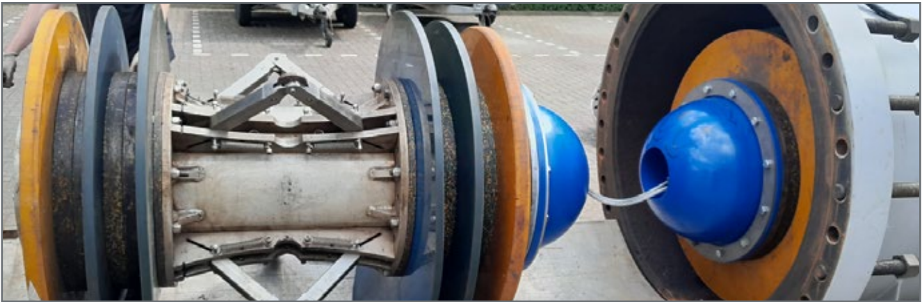
Figure 3: Loading of the bidi & inspection tool during the test
