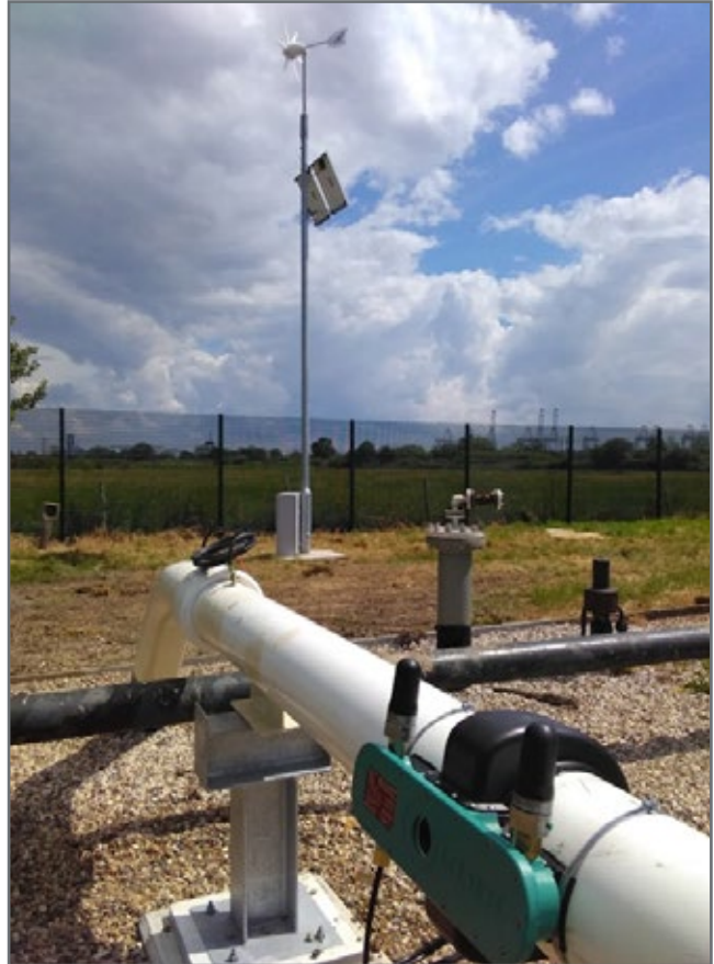
Figure 1: Atmos Eclipse powered by wind and solar
