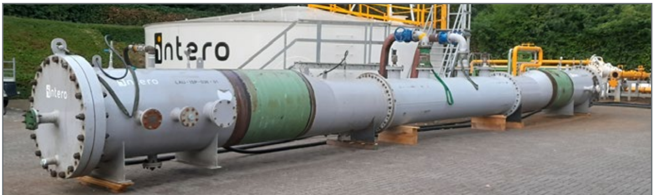
Figure 2: The test spool piece and extended pig traps.
