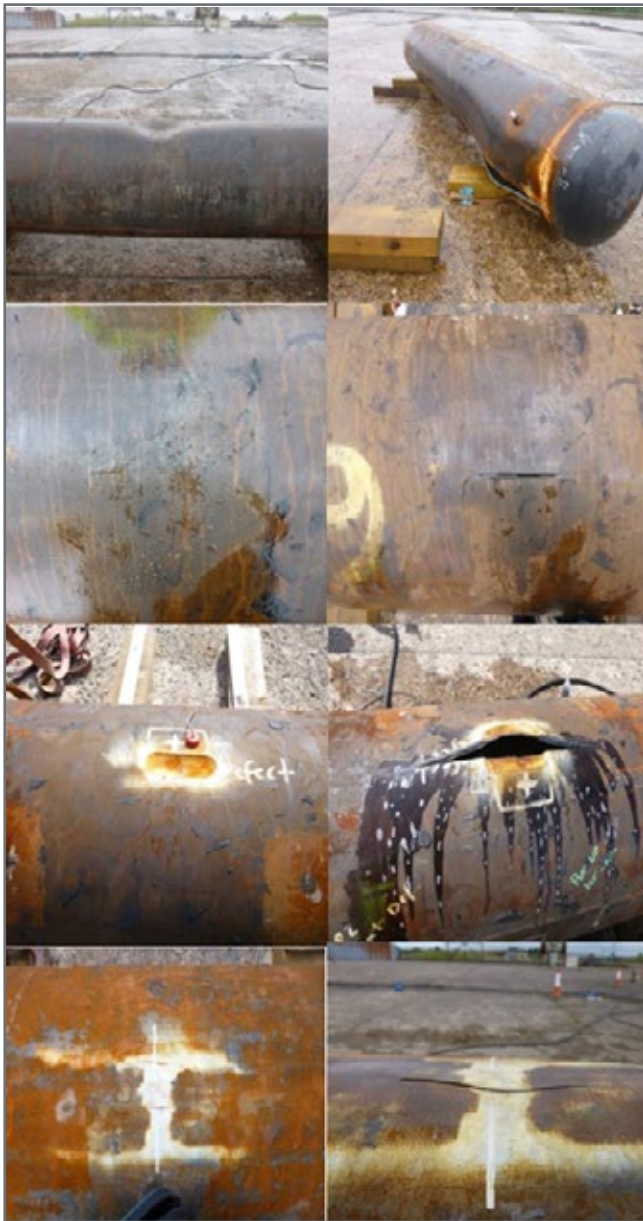
Figure 17: Hydrostatic Burst Test Defects (before and after test)
