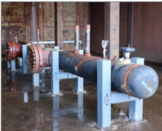
Figure 18: WP1 Tee Fatigue Test Vessel
