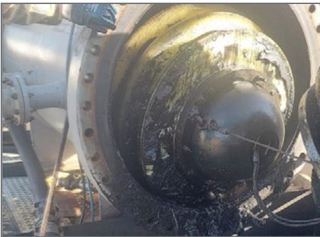
Figure 6: A brush pig being removed
