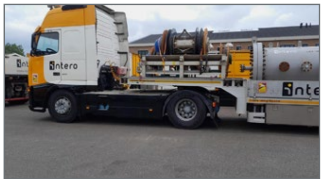
Figure 5: The transport with Ili tool, launcher / receiver, hoses etc.
