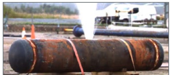
Figure 15: Hydrostatic Burst Test
