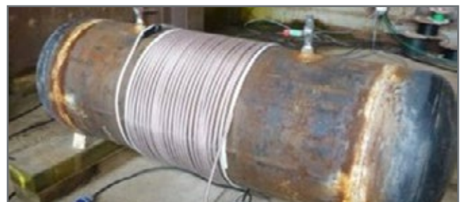
Figure 16: Heating of defect on hydrogen burst test vessel
