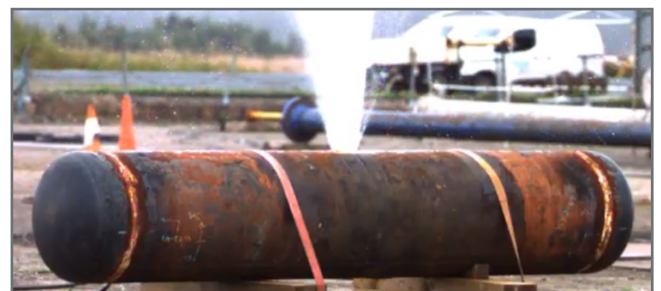
Figure 15: Hydrostatic Burst Test
