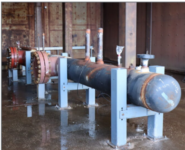
Figure 18: WP1 Tee Fatigue Test Vessel
