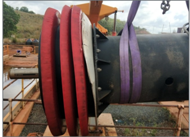
Figure 6: Damaged gauging plate
