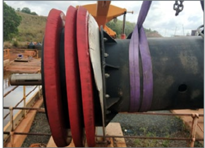
Figure 6: Damaged gauging plate
