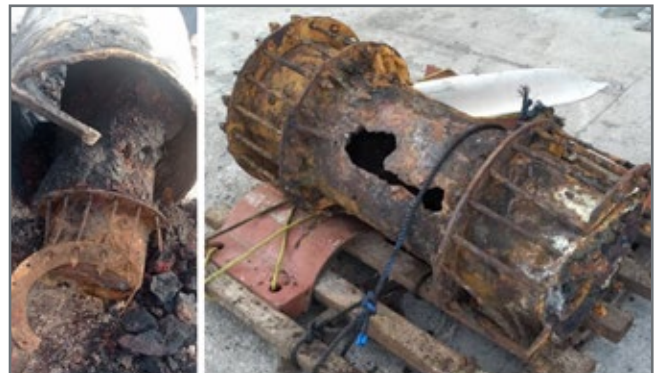
Figure 15: Recovered Stuck Pigs from Damaged Location (Third and Fourth pigs of first Dewatering Operation) [5]
