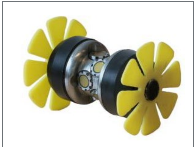
Figure 7: The miniaturised intelligent pig. This is the 4th generation of single body ultrasonic intelligent pigs.
