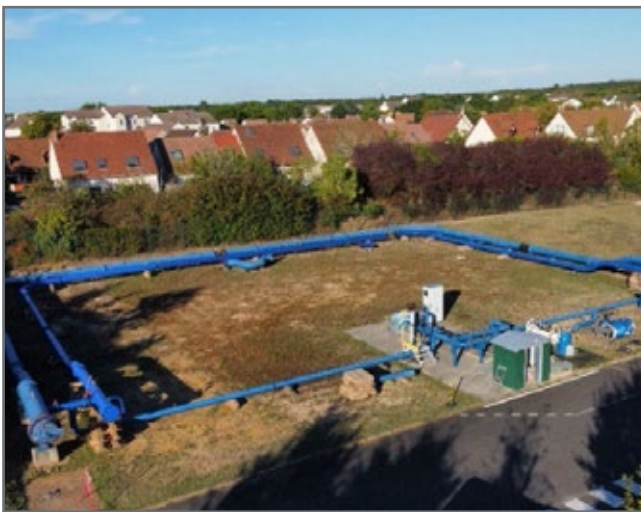
Figure 10: Trapil's 12 and 20" test spools
