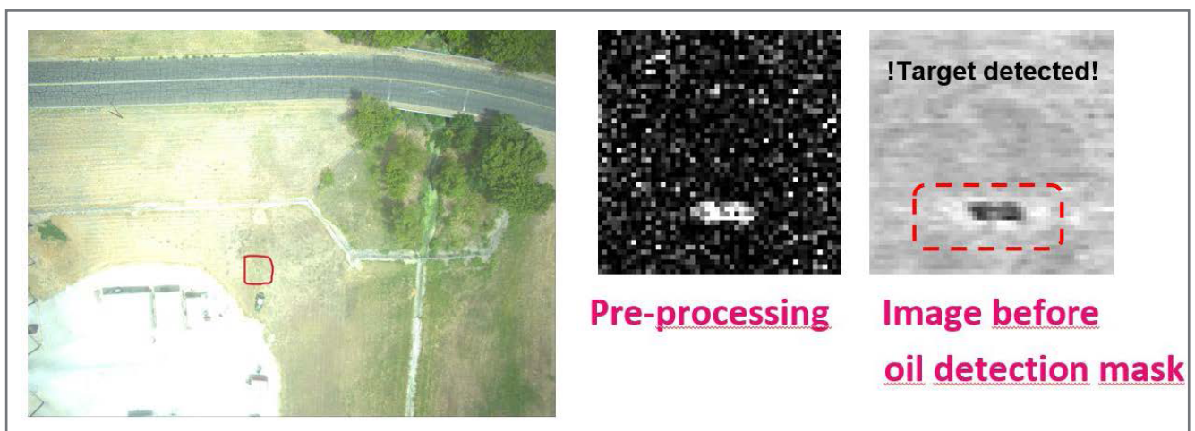
Figure 11: Testing site with diesel mixed in soil with vegetation detection results of the preprocessing and just before applying the hydrocarbons detection algorithm
