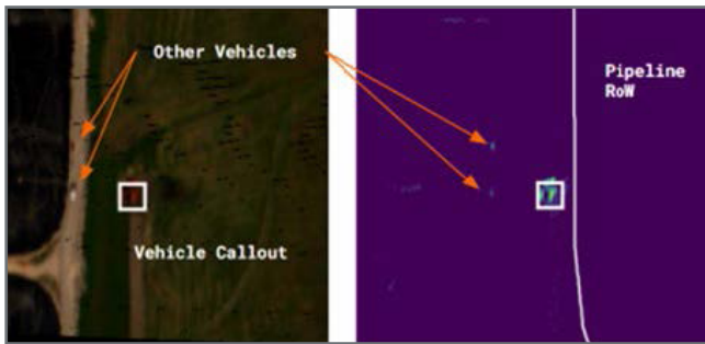
Figure 6: Aerial Detections of vehicles identified along a Pipeline Right of Way. This Detection has used Geofencing to automatically exclude vehicles traveling a public Roadway.
