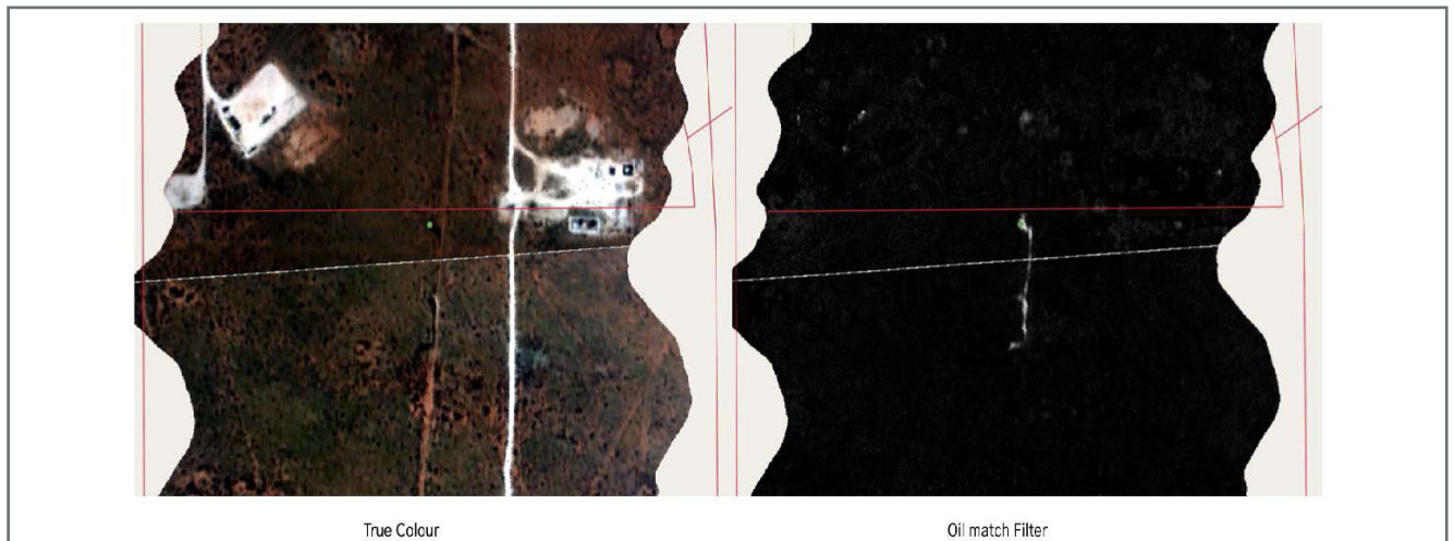
Figure 5: A detection of Hydrocarbon in the soil spilled along an Operator Asset. This figure shows our data in the True Colour Image, Google Earth Imagery for Scene Context, and the Detection Map of the Oil Matched Filter.
