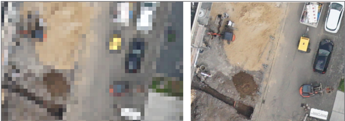
Figure 4: Example of image resolutions. Left 50cm p. Pixel (GSD), right 5cm GSD, taken by manned aircraft.
