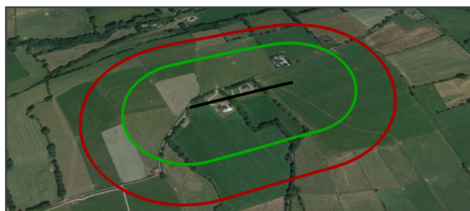
Figure 5: Standard Escape Distance – Methane (red) vs Hydrogen (green) (ID = 0.7m, 70 bar)
