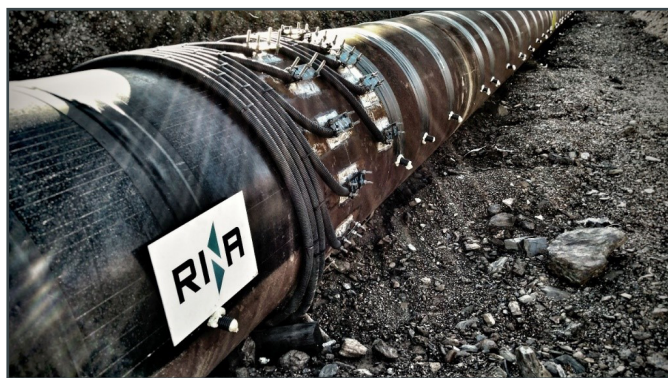
Figure 6: Test line fully instrumented
