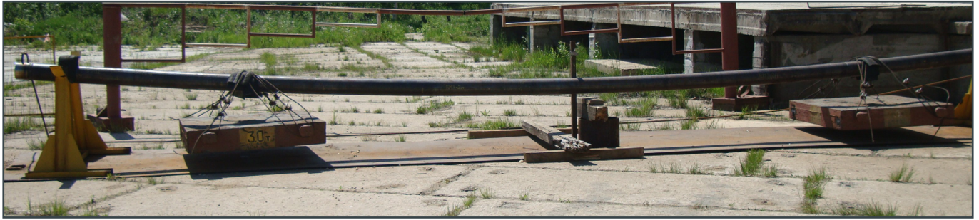
Figure 5: HFW combined load test (courtesy of JSC VSW (part of OMIK))
