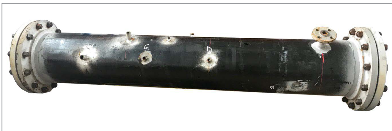
Figure 6: Tube comprising the typical illegal tapings
