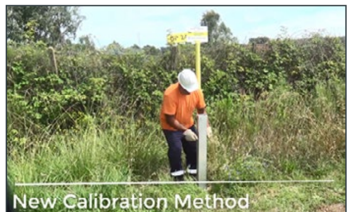
Figure 9: The falling mass calibration device
