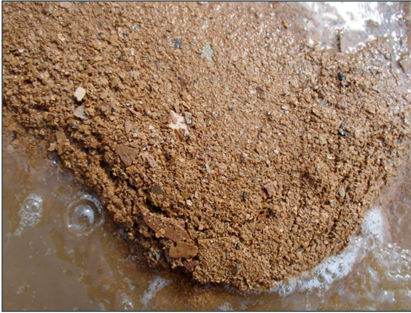
Figure 7: Picture Showing Crushed Scale Chips after the Third MCT Cleaning Run in a 14" Brine Water Pipeline
