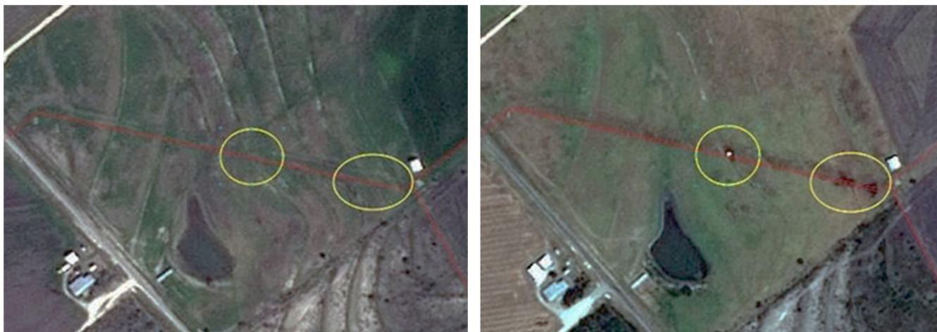
Figure 2: February 9, 2015 (left) and August 10, 2015 (right). The yellow ovals indicate areas of leakage confirmed by the operator
