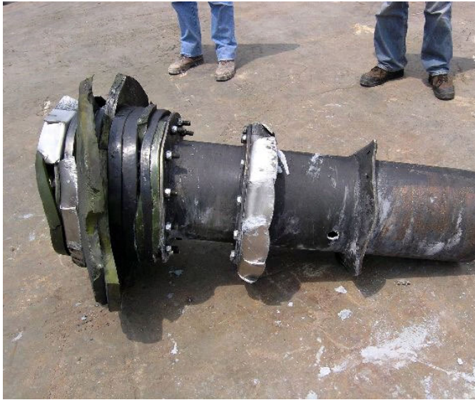
Figure 3. Damaged gauge pig and CCTV inspection results
